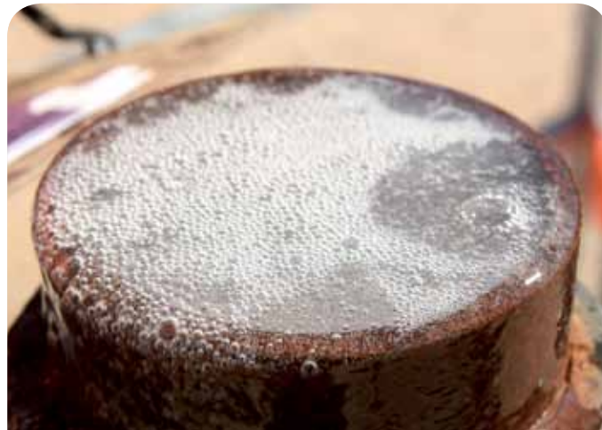
Naturally occurring methane can be seen producing bubbles in a groundwater monitoring bore — this bore is located in an area where CSG production is not yet taking place.
