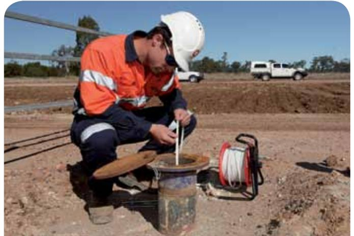
Measuring water levels in a monitoring bore
