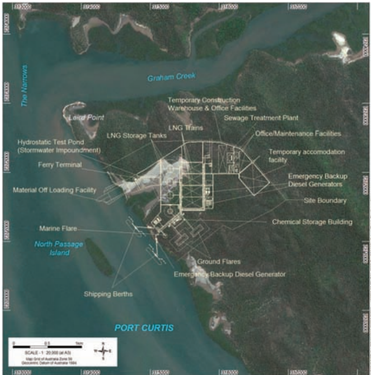
Figure 22.5 Indicative site plan for the LNG facility
